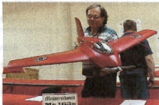
Paul Weigand ME163B KOMET, Supertigre .61 ABC with MACS pipe, wing slots, droppable undercarriage, center chord flaps
