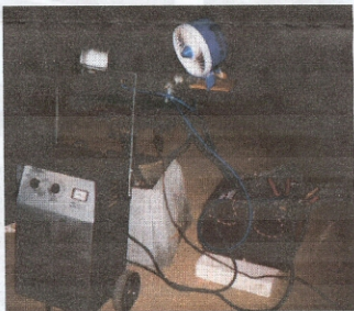
motor, fan, concrete stand, two batteries, charger
